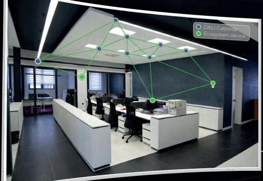
Standardized gateways allow existing DALI wired products to be used in either Bluetooth® mesh or Zigbee® wireless ecosystems. Gateways translate between protocols, and DALI control gear can report luminaire, energy and diagnostics data to the wireless network.
